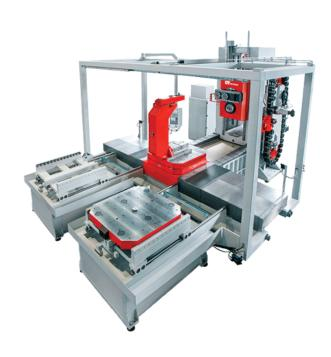
Equipped with two tables. Supports up to 6000kg on each pallet.
